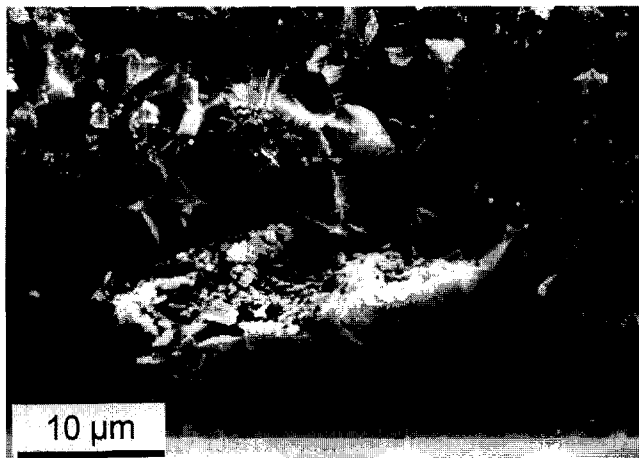
Fig. 14. SEM micrograph of a typical processing flaw in nanocomposites on a fracture surface near the tensile surface.
