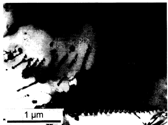
Fig. 13. TEM micrograph of an \text{Al}_2\text{O}_3/5\ \text{vol}\% \text{SiC} nanocomposite showing dislocation networks (courtesy S. Jiao).
